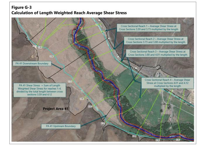
The average energy grade slope was calculated using the same array of cross sections, all of those that fall within the project area, as well as the cross sections immediately upstream and downstream. The energy grade elevation at each cross section at the upstream and downstream ends of the project area was differenced and divided by the total length to determine the energy grade slope for the project area.
